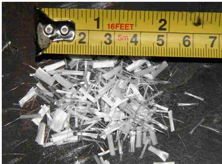
Figure 2-7: Kuralon RECS 15x8mm polymer fibers.
