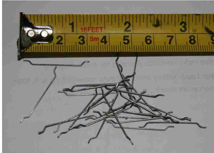
Figure 2-6: Dramix ZP 305 steel fibers.
