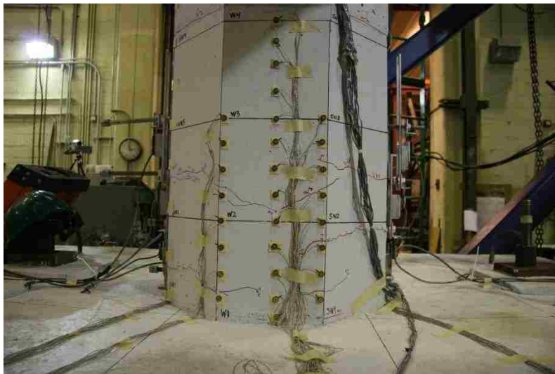
Figure 4-3: PreT-SS after cycle 5-2 when first residual crack was observed.
