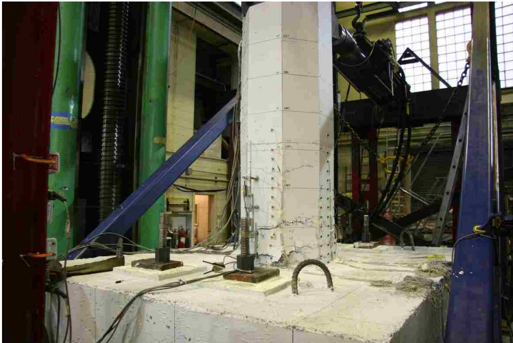
Figure C - 3: Column fully spalled, cycle 9-1.
