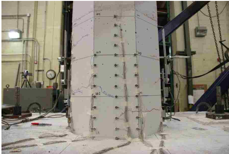
Figure 4-2: PreT-BS after cycle 4-1 when first residual crack was observed.
